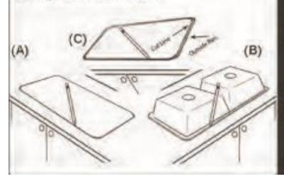
Support the cutout until the cut is complete or it could cause damage to the countertop.
